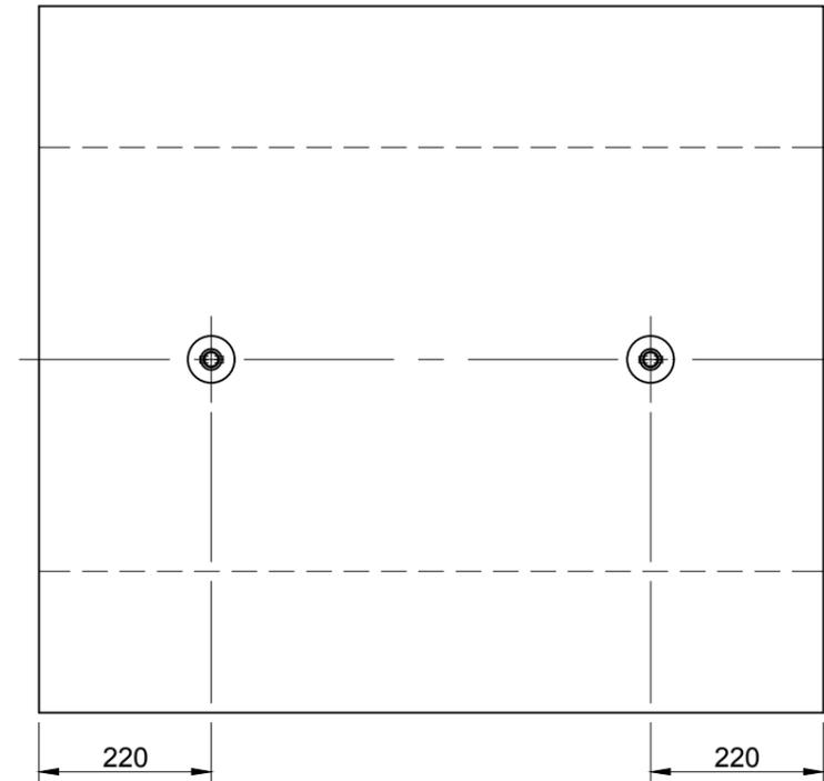
Recess Socket for M20 Nailing Plate.
