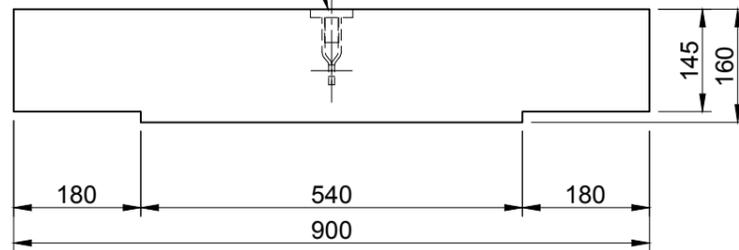
M20 Flat End Lifting Socket
